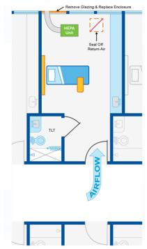
Figure 2. HEPA filtered to outside.
