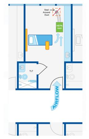
Figure 4. HEPA filtered to return air.
